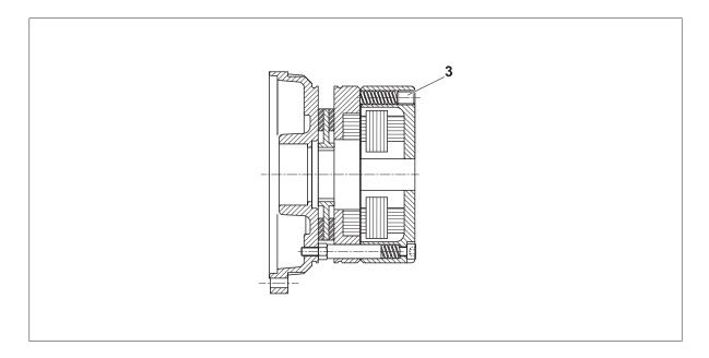
Brake torque can be adjusted steplessly by changing the preload of springs (3).
