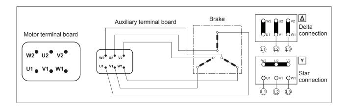
Wire the brake according to voltage and type of connection as shown on motor name plate.
